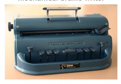
The Perkins Brailler is a solid mechanical 6-dots-braille writer. It is equipped with adjustable margin stops left and right, backspace and line-switch key, key lock at line end and a bell for acoustic signal 7 characters before line end. The Perkins Brailler is a single sheet Brailler. Due to its integrated handle it is easy to carry. The housing is made of aluminum with enamel baked on to protect it.
