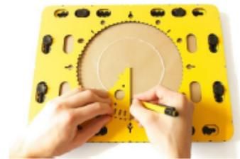
The TactiPad is a versatile drawing board which enables a VIP (Visually Impaired Person) to make a tactile drawing themselves or on which someone can make a drawing for the VIP. These drawings are made on a thin sheet of plastic foil on top of a layer of rubber. By firmly pressing down on the foil the lines will raise instantly, forming the tactile image. The ergonomic design makes drawing easier and much more enjoyable.
